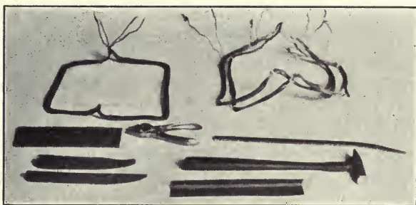
FIG. 123.—At top, one whole and two damaged Eickemeyer coils taken from an elevator motor. At bottom, fiber drifts, slot insulation, hammer, parallel jaw pliers and coil lifter.
